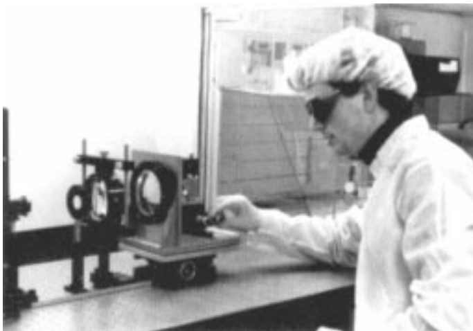
Prototype 'Half-Field Dyson' optical system, emphasizing the compactness and simplicity of this approach (photograph courtesy of A. Walther).
