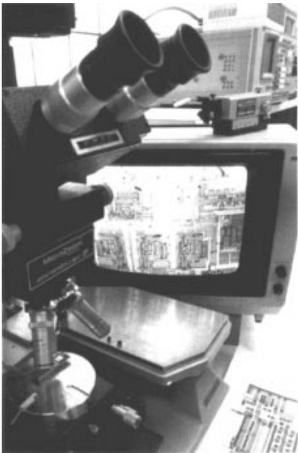
*Testing phase of chips for research at the Ohio State University on analog CMOS/BiCMOS standard cells for VLSI signal processing applications under the direction of Professor Mohammed Ismail.*
