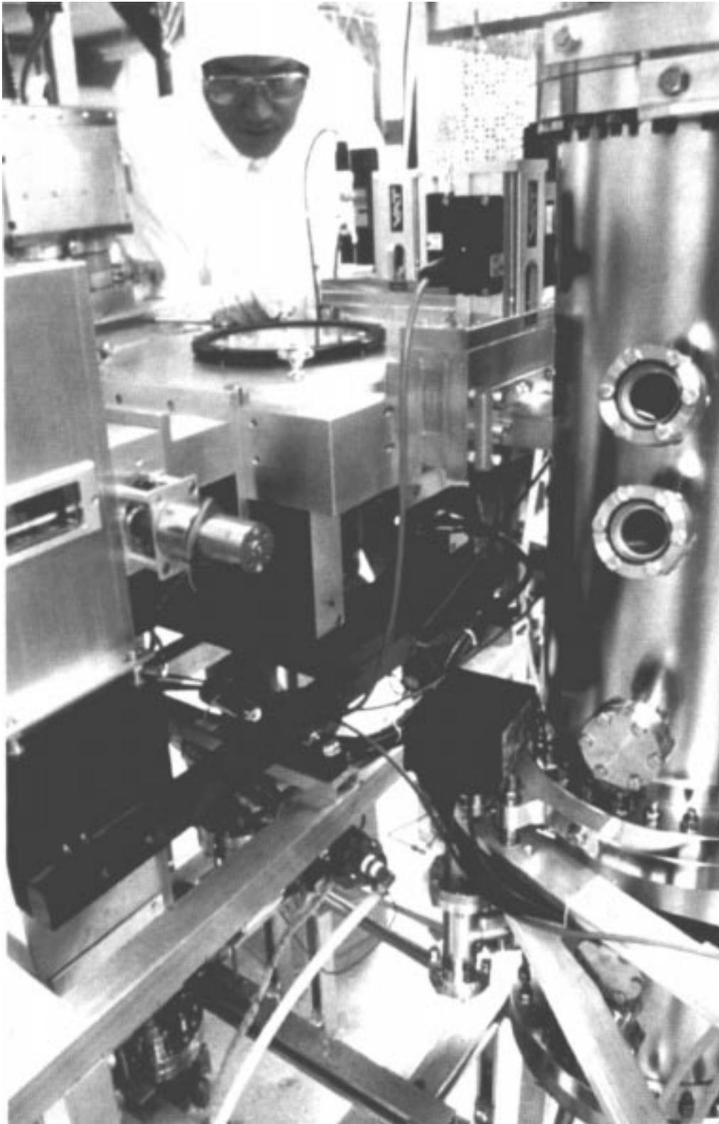
*Graduate student examines central wafer handler of North Carolina State University's cluster tool for low-thermal-budget, single-wafer, in-situ processing.*
