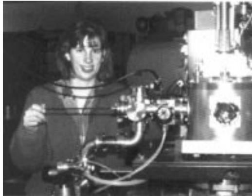
Cornell graduate student Nancy Stoffel loads polyimide samples into an ion-beam analysis chamber.
