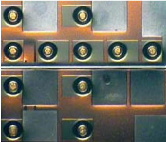
Figure 11. Technology for inductive/capacitive chip-to-package connection
