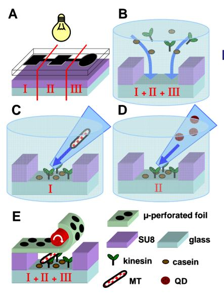
Fabrication of "Smart Dust" devices requires a combination of lithography, fluidic delivery and bonding using hard and soft materials.
