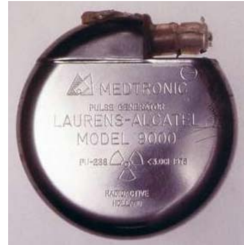
30% of Pacemakers implanted from 1971-75 were radioisotope powered
