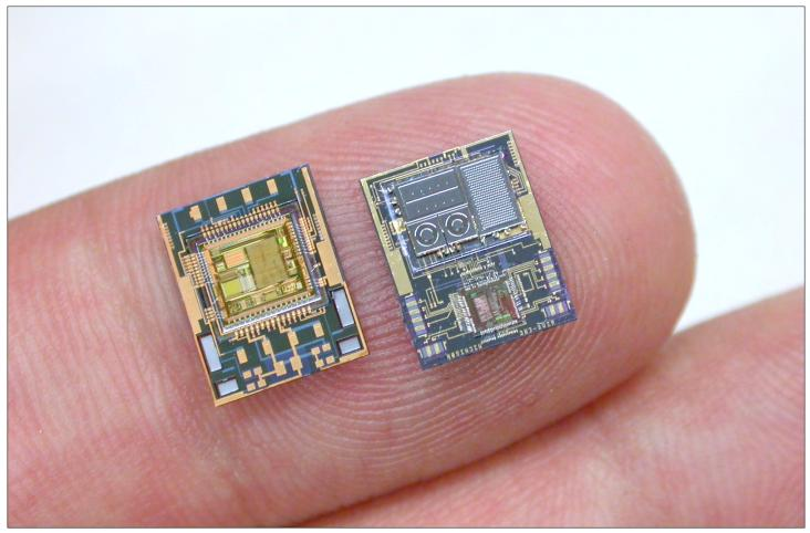
Embedded µComputer, 16Mb Flash Memory, Sensors for Pressure, Temperature, Humidity, and Off-Chip Biosignals
