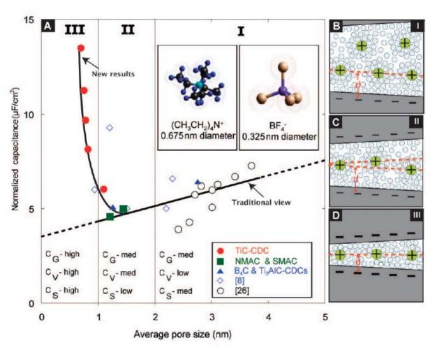
Distortion of solvation shells in sub-nm pores results in enhanced ion storage capacities
