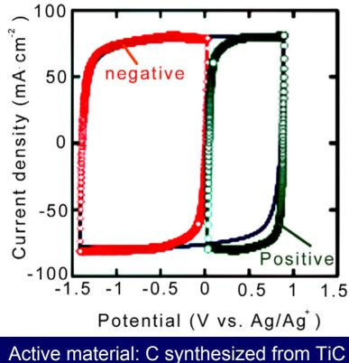
Active material: C synthesized from TiC and having the pore size of about 0.72 nm Cyclic Voltammogram taken at a scan rate of 20 mV/s in 3 electrode cell configuration
