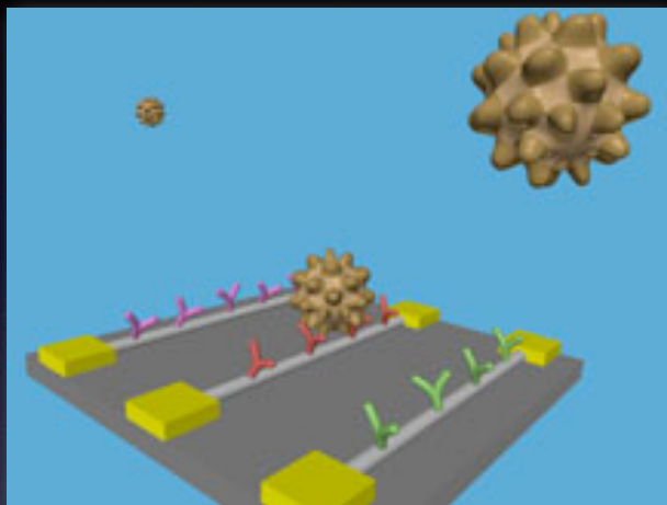
Nanowire transistor arrays detection of viral particles (C. Leiber, Harvard University)
