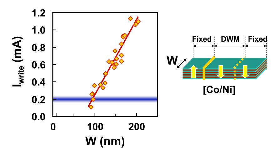
At less than 100 nm width, the write-current becomes less than 0.2 mA.  $\Rightarrow$  The most important criterion is satisfied.
