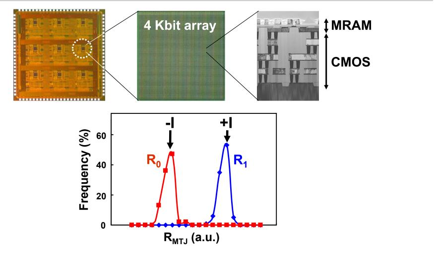
The two resistance states of the MTJ are clearly separated. The change of resistance is consistent with current direction.
