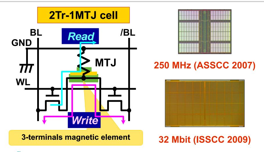
No problem with either write disturbance or read one ⇒ Great advantage for high-speed operation
