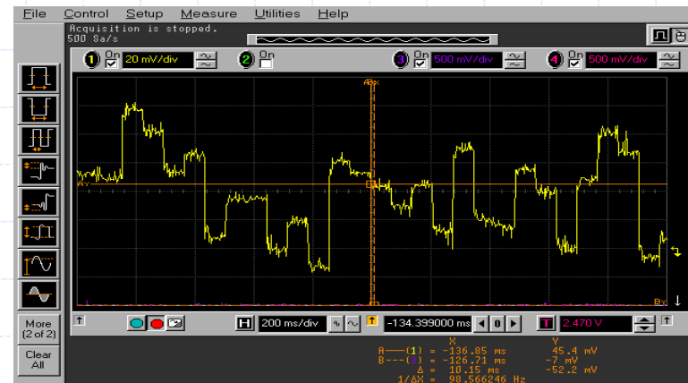
Waveform illustrating V_{TH} variation across multiple devices
