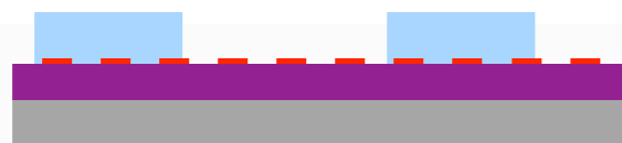
PMMA cylinders shown after NIL
