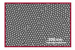
(2) Imprint of Template into PMMA
