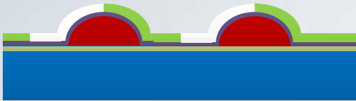
F. Electroplating Mold Patterning
