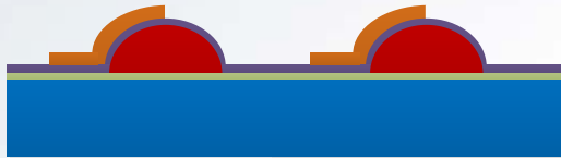
G. MFIs Formation Using NiW Electroplating
