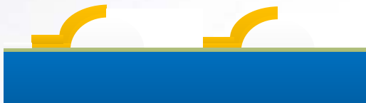
I. MFIs Releasing and Gold Passivation
