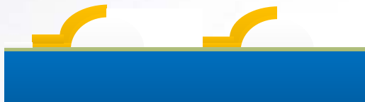
I. MFIs Releasing and Gold Passivation
