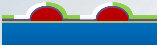
F. Electroplating Mold Patterning
