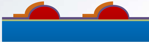
G. MFIs Formation Using NiW Electroplating
