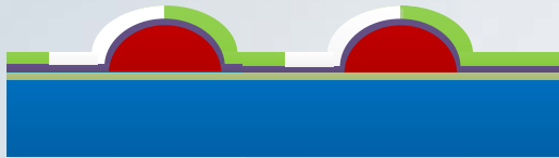
F. Electroplating Mold Patterning
