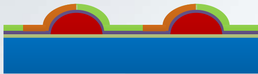
G. MFIs Formation Using NiW Electroplating
