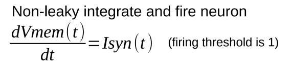
Exponentially decaying synaptic current  $Isyn(t) = \sum_{i} w_i \exp(-(t-t_i))\Theta(t-t_i)$  $\Theta(t-t_i)$ : Step function
