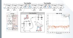
**Highlight:** designed a single channel ADC achieves a 56dB SNDR at ~5GHz input frequency, and 52dB SNDR at ~10GHz input frequency, with a power consumption of 27mW.
