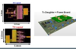
**Highlight:** designed and taped-out a PAM-4 50Gb/s transmitter and two versions of receiver in Intel 16nm targeting a FOM of 90 fJ/b/dB
