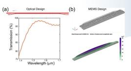
**Highlight:** developed a new silicon photonic MEMS design that is compatible with AIM Photonics process stack, and taped-out an 8x8 switch prototype
