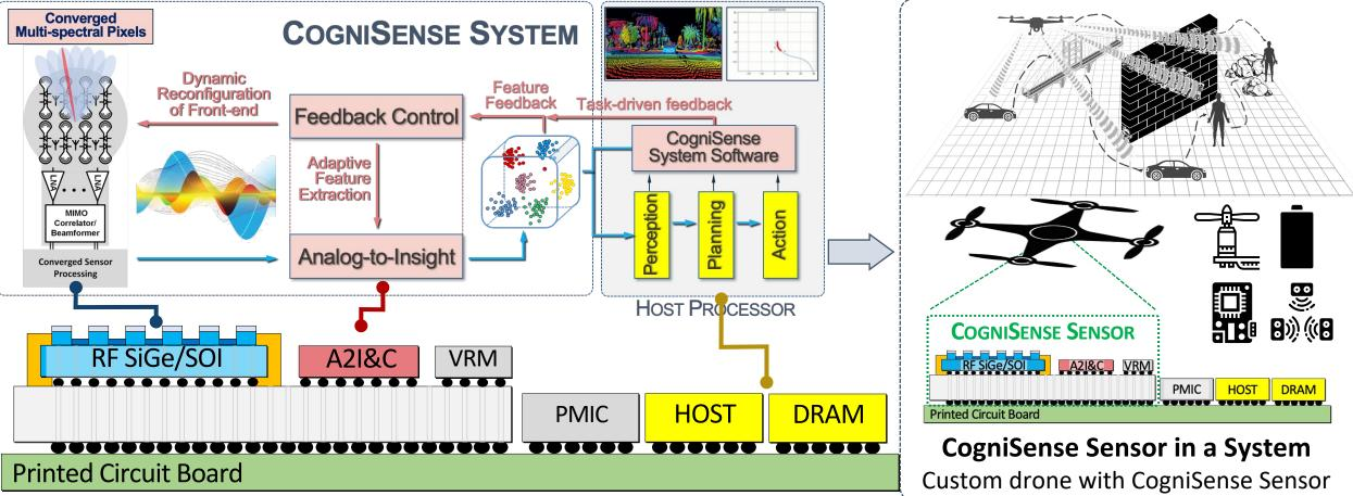
Cognitive multi-spectral sensors directly generate trustworthy insights from wideband multimodal analog signals using closed-loop feedback control of the sensor hardware and feature extraction algorithms that enable energy-efficient sensing-to-action.
