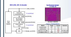
**Highlight:** designed a harddecision decoder achieving energy-efficiency of < 0.5 pJ/b at a single channel throughput of 37 Gb/s and a coding gain of 5dB in Intel 16 (Tape-out -December'23)
