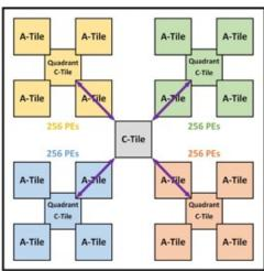
Conceptual sketch of a configurable chiplet architecture
