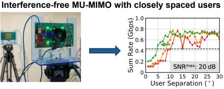
IBM 28-GHz PAAM connected to USRP SDRs
